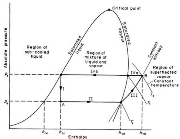
Fig. 2. Refrigeration P-H Diagram
