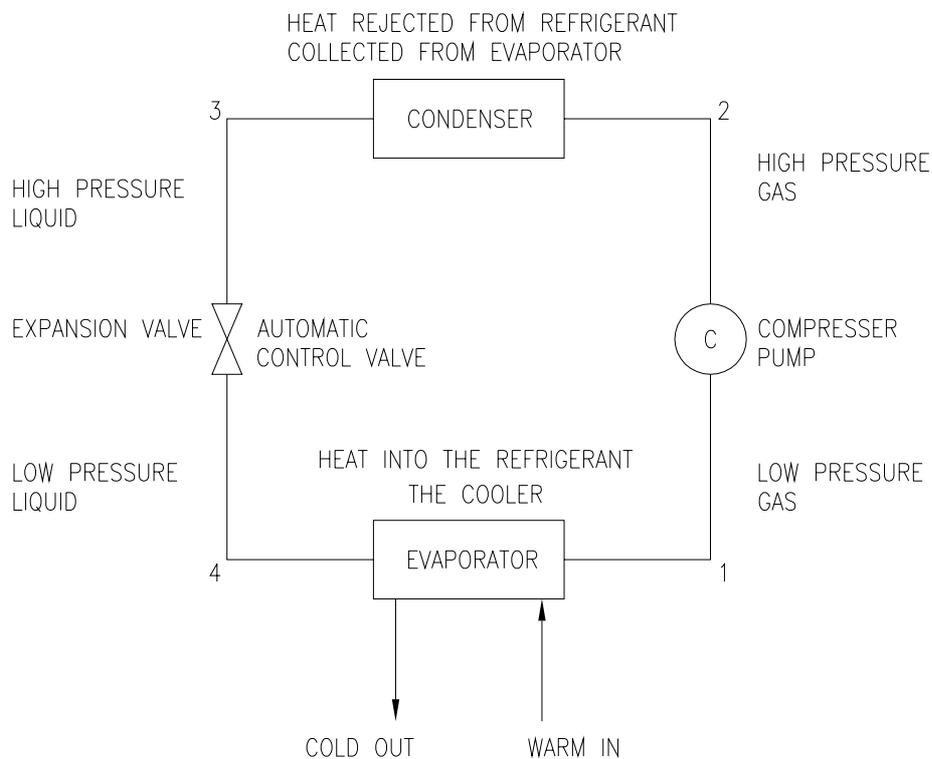
Fig 6. The Refrigeration System
